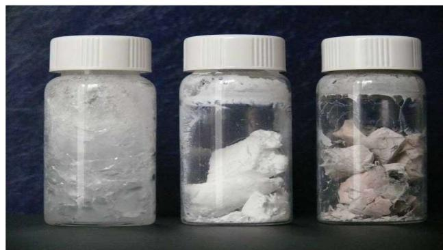
Products obtained after each of the three main steps for preparation of SAP matrix
